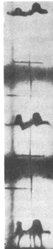
Fig. 4. Deformation and breakup of drops in constrained conditions.
